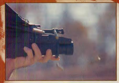
Cases tumble out of the F2000 in several full-auto bursts. Note the absence of muzzle rise in this very well-balanced and controllable weapon. (right) A magazine of 5.56mm ball and a 40mm TP round ready for fun in the sun.
